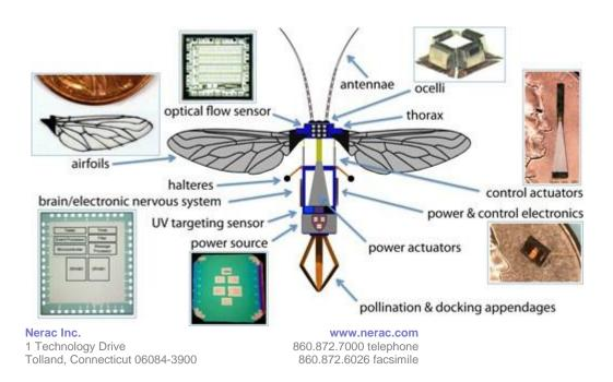
A MAV bee using a biomimetic ocelli senses light levels with four phototransistors to estimate the angle orientation relative to vertical; optic flow micro sensors to measure the MAV perceived motion and provide information for collision avoidance, altitude and landing; and biomimetic antennae for rapid feedback of wind velocity. Robobees: Harvard School of |Engineering and Applied Sciences.
